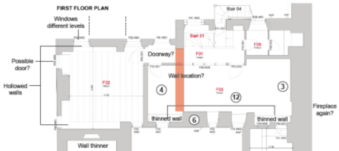
Figure 4 CFA - Irregularities of First Floor of the Northern Block
