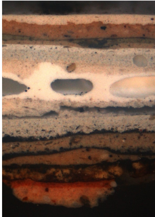
Figure 60 Sample 11 - Cross-section of paint from detached shelving x100
