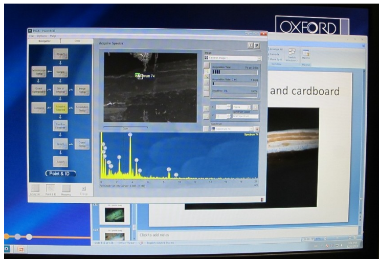
Figure 63 SEM image with elemental spectrum
