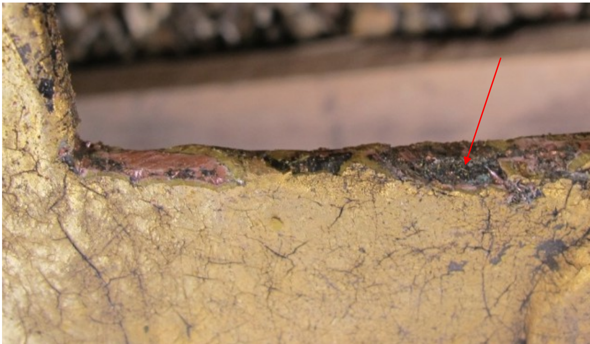
Figure 16 Sample 15 - Traces of early decorative schemes visible beneath pink primer
